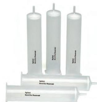
Empty SPE cartridges with two frits (pre-inserted),
