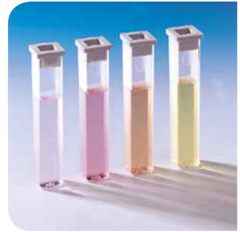
Plastic cells, frosted on two sides, volume 10 ml, path length 13.5 mm, with lid
