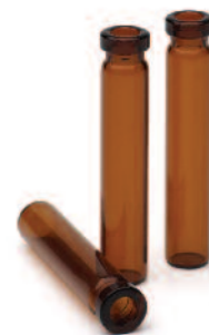
Amber, flat bottom crimp top micro vials, 8010-0153
